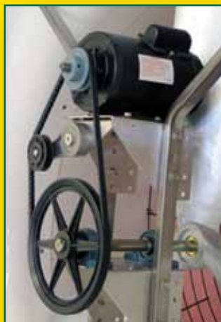
Motor mount and drive assembly utilize a rugged box frame design to increase motor life.
